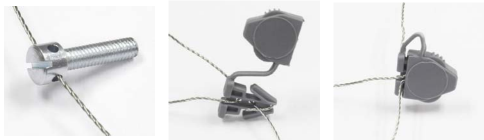
Figure 2-84: Use of the Sealing Kit: Wire Through Screw (left), Wire Through Seal (center), Seal Closed (right)
