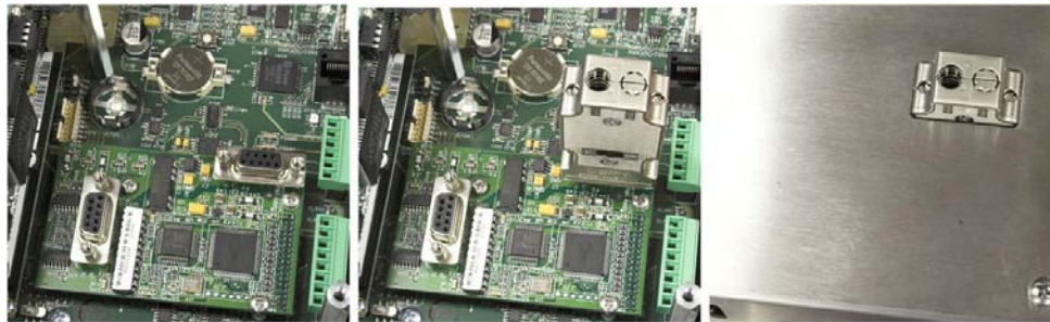
Figure 2-67: PROFIBUS PLC Module Connector for Panel Mount Enclosure
