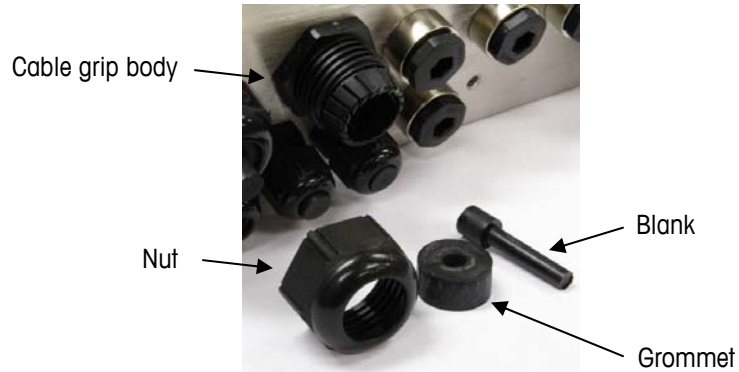
Figure 2-22: Cable Gland Components
