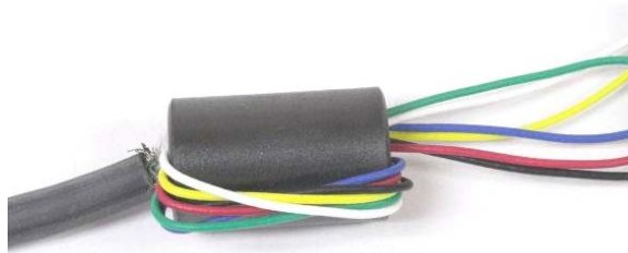
Figure 2-16: Ferrite Core on Analog Load Cell Cable
