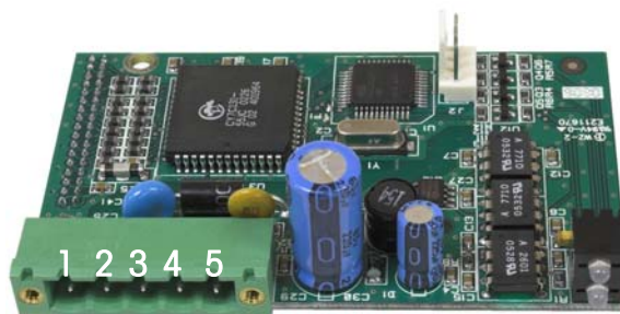
Figure 2-62: DeviceNet Option Board Connector Pin Numbering
