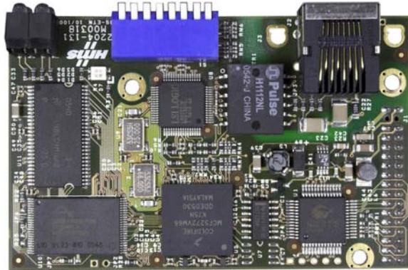
Figure 2-72: Ethernet / IP PLC Module
